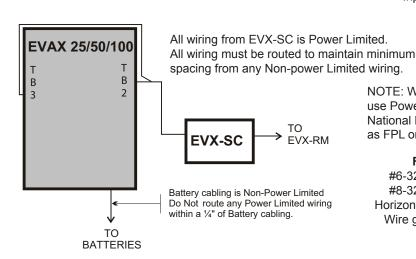
NOTE: When circuits are Power Limited. use Power Limited cable as detailed in the National Electrical Code, Article 760, such as FPL or FPLP type cabling.
