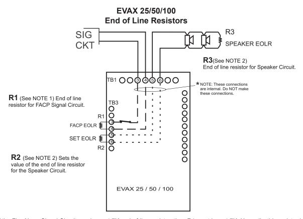
**NOTE 1:** If the Fire Alarm Signal Circuit requires a 4.7K end-of-line resistor, then R1 must be a 4.7K. Normally, this resistor is connected to the Signal Circuit through a closed Common Trouble contact. When the EVAX 25/50/100 goes into Trouble, the contact opens, producing an "Open" on that Signal Circuit and notifying the FACP.
