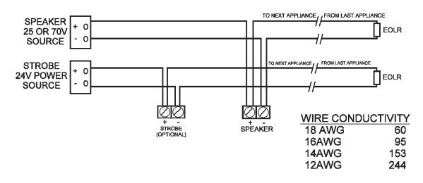
NOTE: DO NOT USE LOOPED WIRE UNDER TERMINALS. BREAK WIRE RUN TO PROVIDE SUPERVISION OF CONNECTION.
