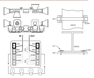
IF THIS CLUSTER IS THE LAST DEVICE ON THE CIRCUIT, PLACE END OF LINE DEVICE ACROSS THE "OUT" TERMINALS, ACCORDING TO CONTROL UNIT MANUFACTURER'S INSTRUCTIONS.
